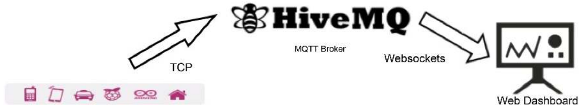
Figure 14. Shows the visualization layer components. It shows how the web dashboard gets the data from MQTT broker (Hive MQ) over HTML web sockets.
