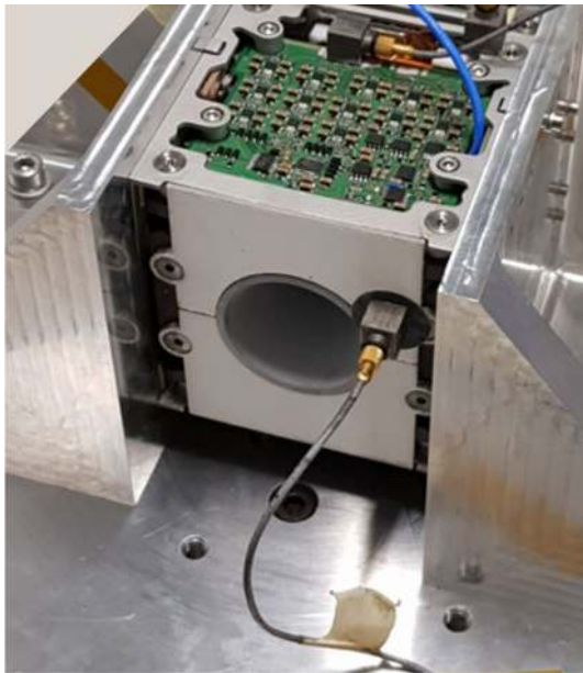
Fig. 4 Mechanical vibration test of the Electro-Magnetic model of REGULUS
