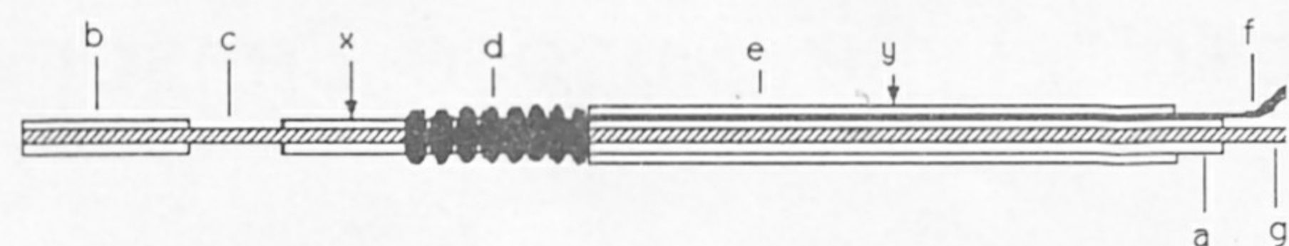
Figure 1. Schematic diagram of the sensor: (a) Teflon-coated Pt-Ir wire (0.25-mm o.d.), (b) Teflon tip, (c) sensing cavity (1-mm length), (d) Ag/AgCl reference electrode, (e) heat-shrinkable tubing, (f) reference electrode terminal, (g) working electrode terminal.
