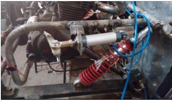
Fig.3 Double acting cylinder for Clutch lever
