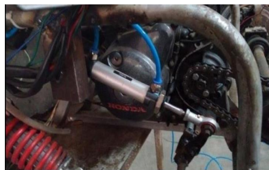
Fig.2 Double acting cylinder for Gear lever
