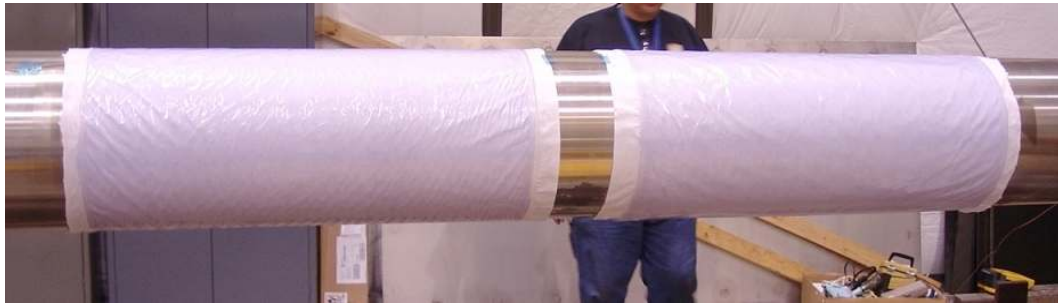
Figure 12. Shells being bagged before cure.
