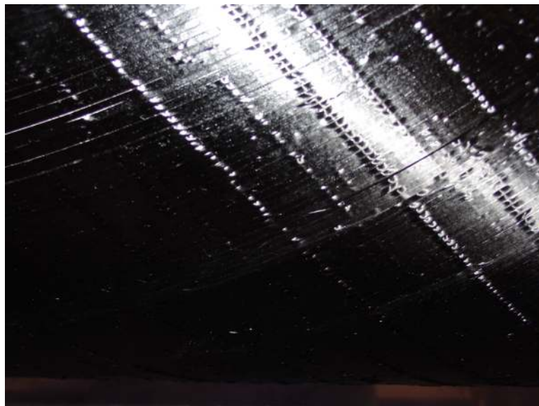
Figure 17. Tow kinking noted during shell fabrication.
