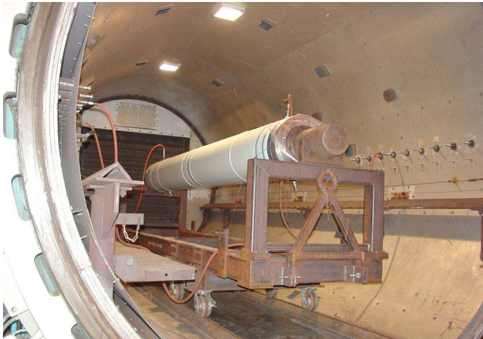
Figure 13. Shells loaded in the autoclave for curing.
