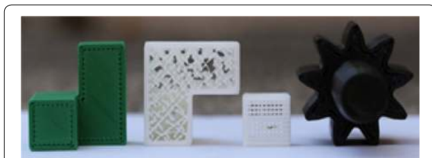
Figure 3 Filling path strategies used in an FDM process
