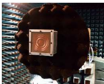
Fig. 8. TA antenna prototype under test in the anechoic chamber.
