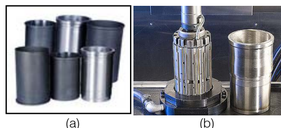
Figure 1 (a) : Photograph of cylinder liner, (b) photograph of honing tool with cylinder liner
