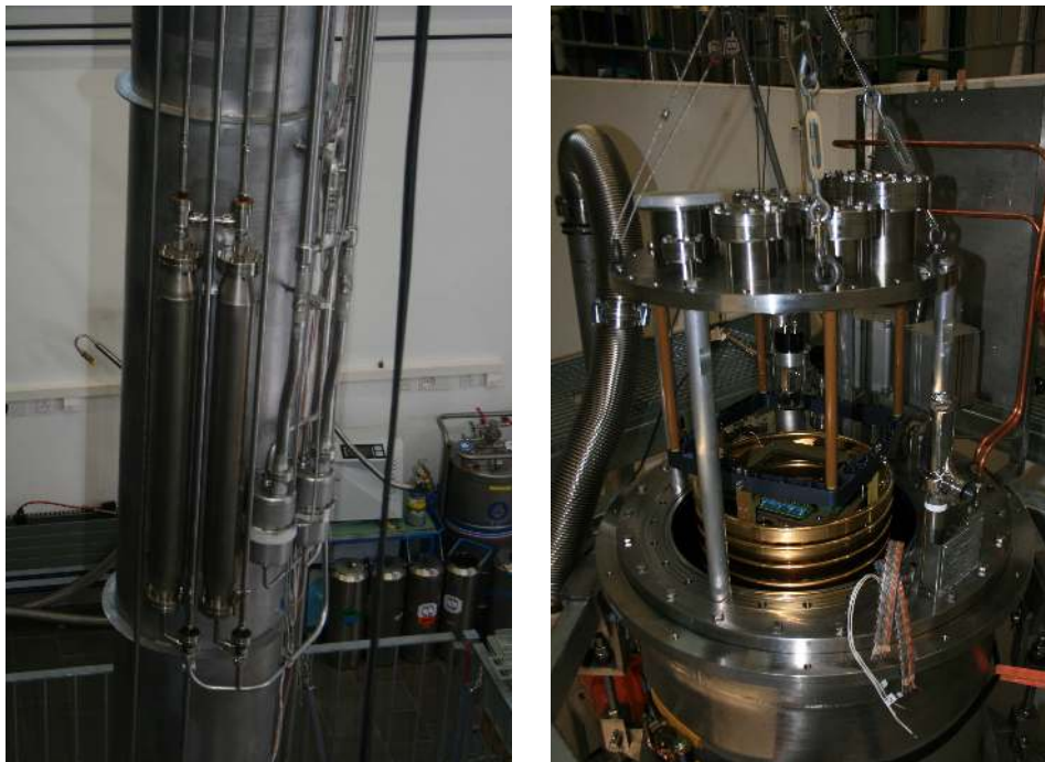
Figure 5. Left: Picture of the inner vessel where the Oxygen-trapping filters and the bellow pump are shown. Right: Picture of the top flange with all feed troughs, field shaping rings, some details of the fastening system to the top flange and two photomultipliers used as trigger.
