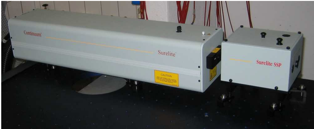
Figure 7. Continuum Surelite Nd:YAG laser with a Surelite Separation Package (SSP) which separates the 266 nm laser beam from all the other harmonics.
