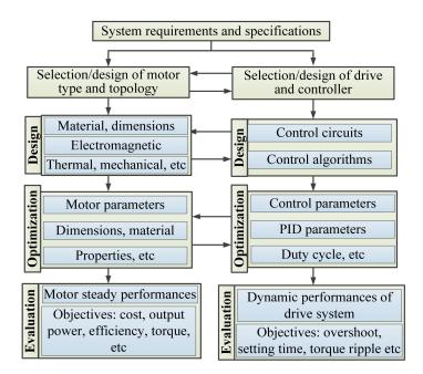
**Figure 8.** System-level design optimization framework for an electrical drive system with specific HSPMM and control system.
