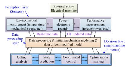
Figure 4. Framework of electrical machine DT modelling process.
