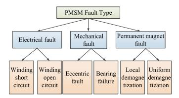
Figure 5. PMSM fault type.
