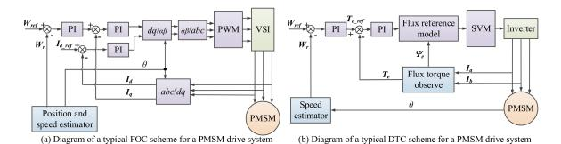
**Figure 2.** Control diagrams of typical FOC and DTC for PMSM drive systems. Note:  $I_d$  and  $I_q$  stand for the d- and q-axis currents, respectively. Ye is the flux, Te the torque. For FOC, the d-axis current is set to zero for achieving the maximum torque per ampere. The current/torque loop and speed loop are set as feedback loops to keep the reference speed  $W_{ref}$  as well as to make a smaller d-axis reference current  $I_{d ref}$ .
