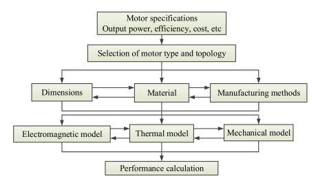
Figure 6. Design framework of HSPMMs and other electrical machines with multi-physics analysis.
