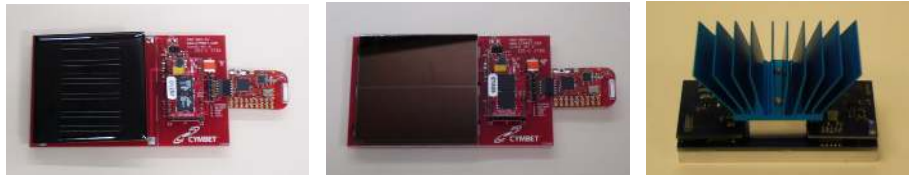
(a) Outdoor Solar Energy Harvester (b) Indoor Solar Energy Harvester (c) Thermal Energy Harvester
