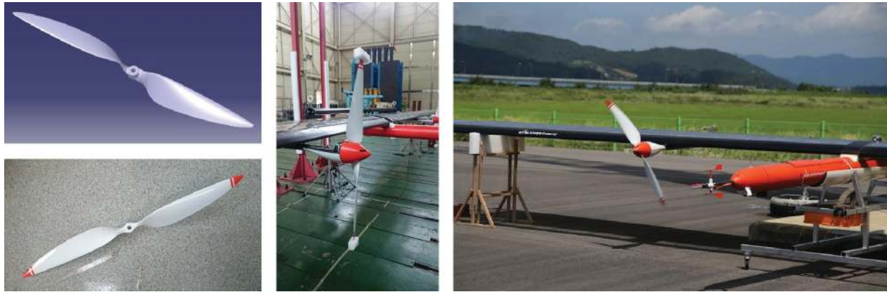
FIGURE 12: Manufactured and mounted propeller for EAV-3.
