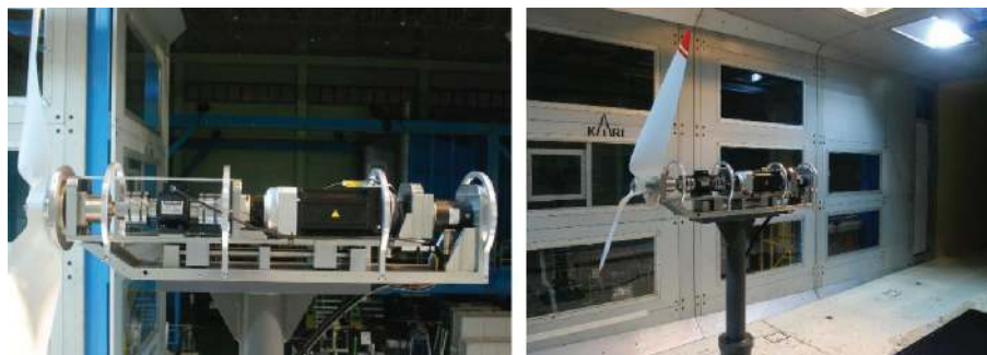
FIGURE 15: Installation of measurement device.
