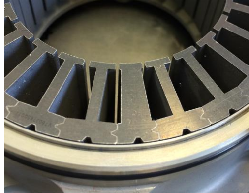
Fig 15. P2 Segments compression fitted into stator housing.
