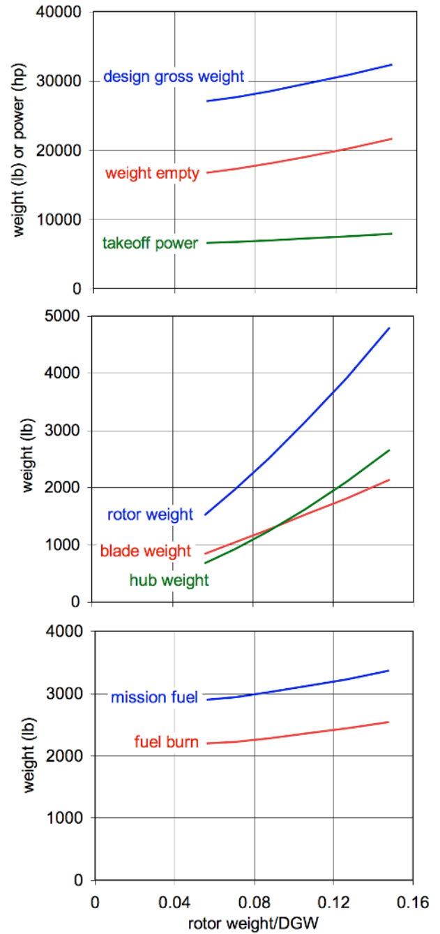
Figure 39. Influence of rotor weight technology (rotor weight fraction of design gross weight) on civil aircraft with regression rotor weight model.
