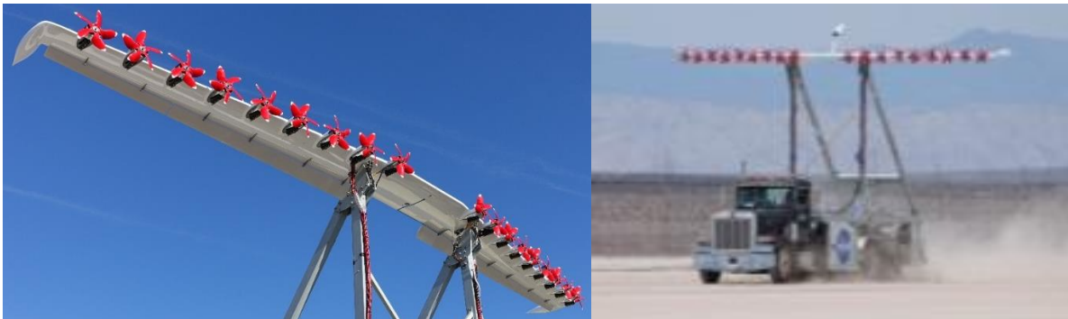
Figure 4: (Left) LEAPTech Wing Configuration; (Right) SCEPTOR Mod 1 High-Lift Propeller Testing at NASA AFRC
