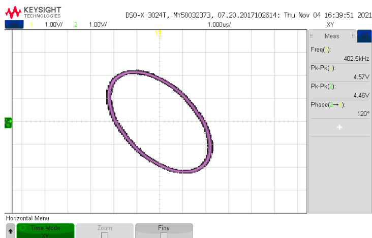
Fig. 22. Lissajous figure of sinusoidal MSO waveforms
