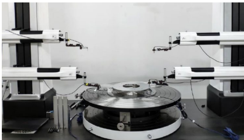
Figure 1. UOI Ultra-precision rotor shape and position error measurement system.
