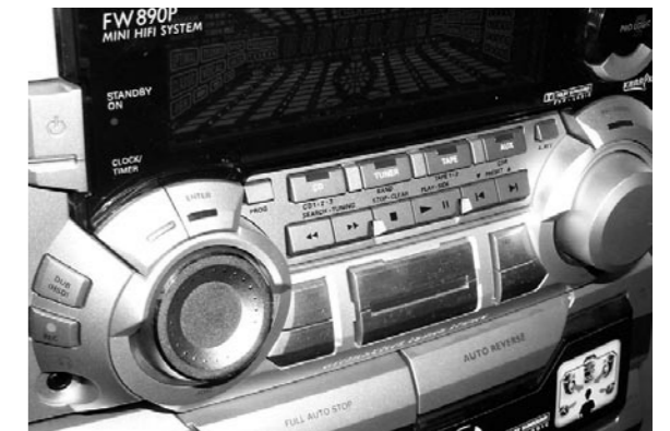
Figure 1: Complexity of visual and physical arrangement of components makes this stereo nearly impossible to decipher.
