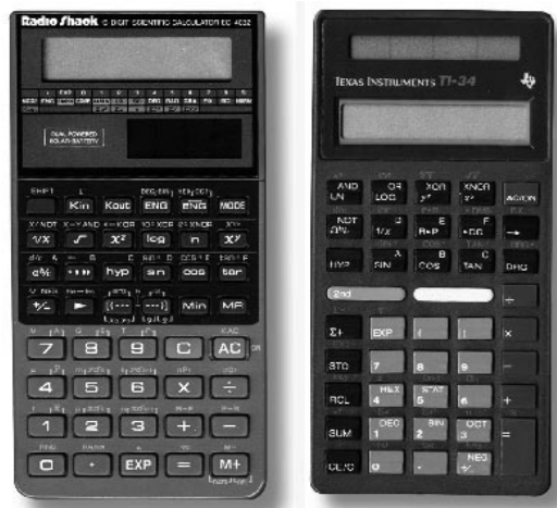
Figure 2: Each calculator has the same functionality, but their form language creates different product experiences.
