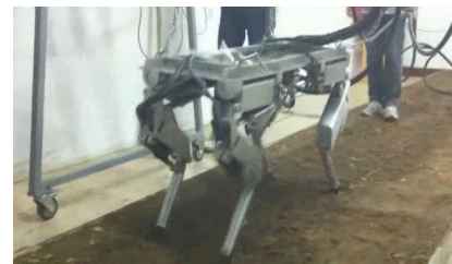
Fig. 14. Scaif-1 trotting on soil ground at 0.4 m/s.
