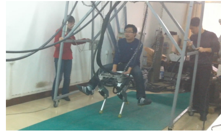
Fig. 13. Scaif-1 trotting with 80 kg payload at 0.4 m/s.
