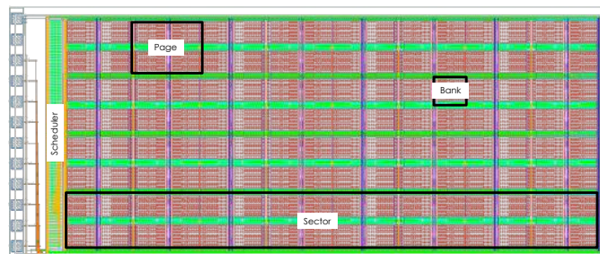
Figure 11: Layout view of the full macro-cell with top analog (right) and scheduler (left).
