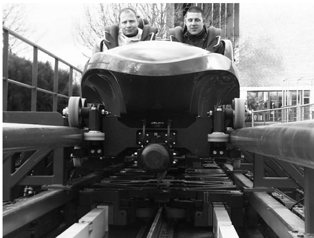
Fig. 19. Linear PM coaster launcher at Six Flags Holland. (Photograph reprinted with the permission of KumBak Coasters.)
