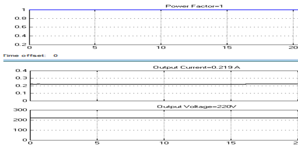
Fig. 7: Graphical Display of Measured I_o , V_o , p.f. parameters.
