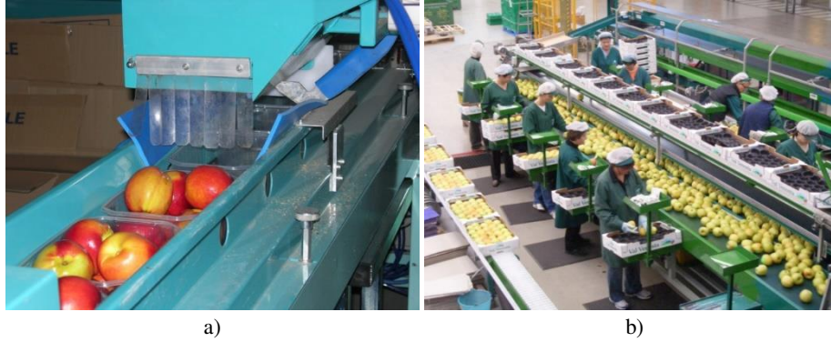
Fig. 1. Examples of packaging lines: a) Automatic packaging line for apples; b) Packaging operations performed by human workers.
