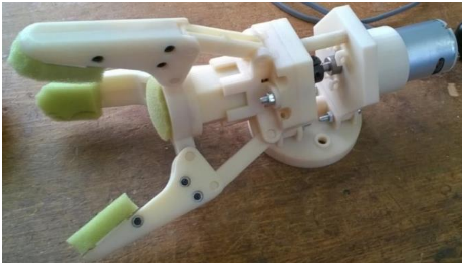
Fig. 5. The gripper prototype built with 3D printing.
