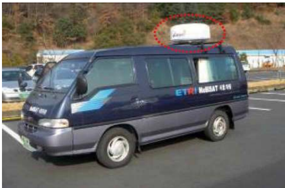
Fig. 16. Antenna system installed on the test van.
