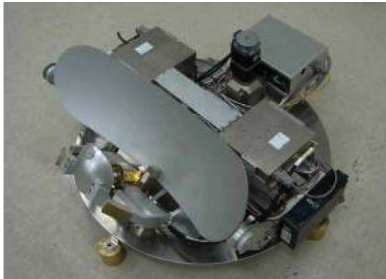
Fig. 12. Photo of the entire assembled mobile antenna system.
