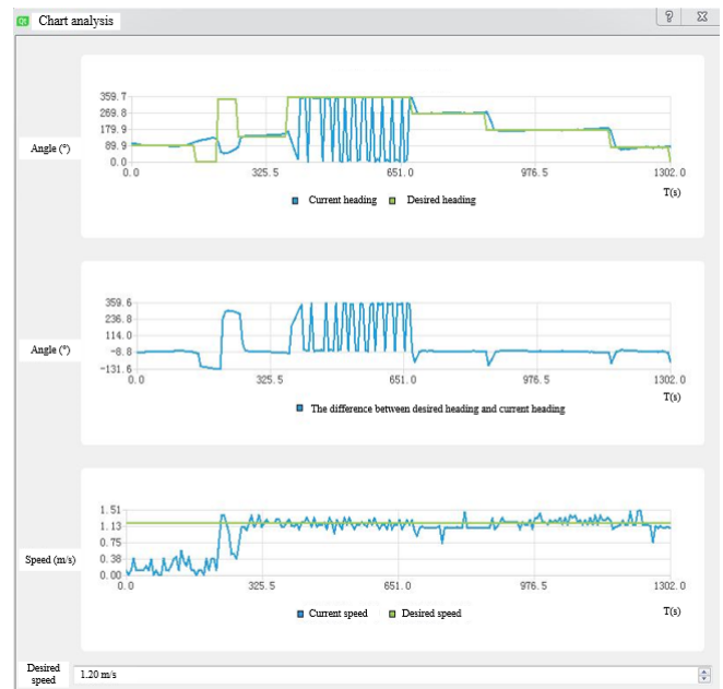
b. Diagram of course and speed tracking.
