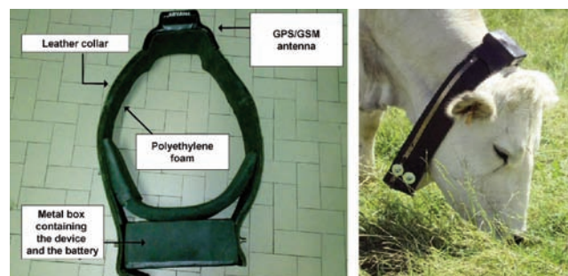
Figure 2. The assembled global positioning system (GPS)-anti cattle rustling and a cow with the antitheft system. GSM, global system for mobile communication.
