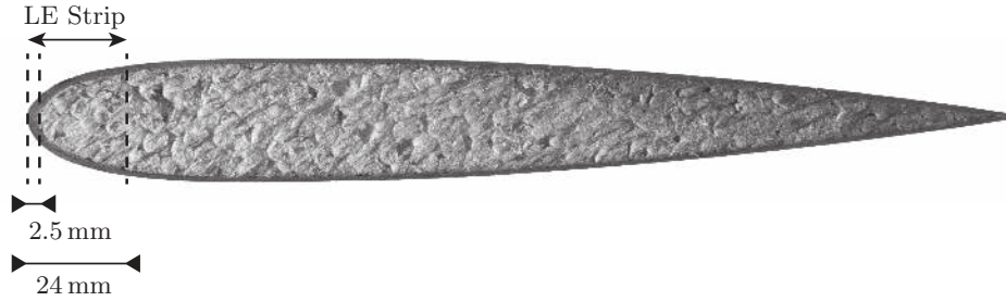
Figure 12: Cross-section of the experimental wing
