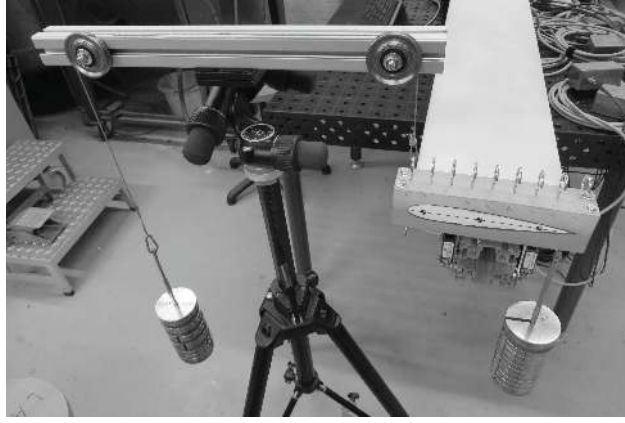
Figure 5: Picture of the structural test setup illustrating an applied tip torque
