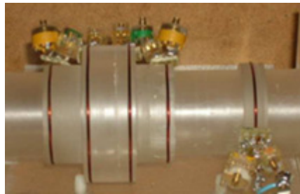
Figure 6. Photograph of the spherical prototype coil
