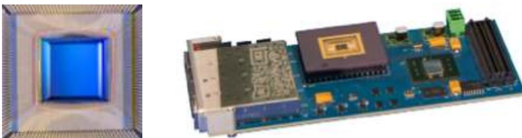
**Figure 7.** Left: protoVIPRAM00, 130nm Global Foundries Low-Power CMOS, 5.5mm X 5.5mm. Right: FMC Test Mezzanine card features a Xilinx Kintex XC7K160T FPGA, 4 SFP+ transceivers, 128MB DDR3, and a 144 pin socket used for testing custom ASIC chips, such as protoVIPRAM00.
