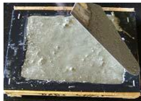
Fig.-6: Concrete filling in mould
