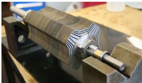
Fig. 15. Prototype rotor lamination stack on the motor shaft before insertion of the stator.
