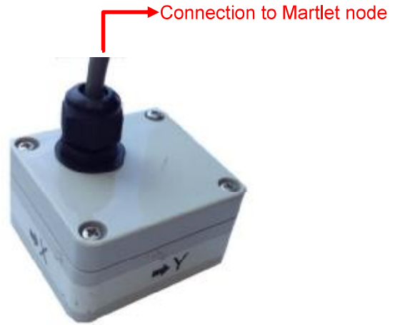
(b) Weatherproof package (2.28in \times 2.52in \times 1.38in)
