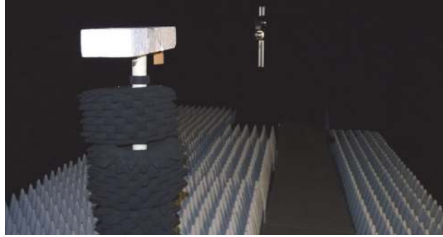
FIGURE 8: Measurement of far-field diagrams in anechoic chamber.
