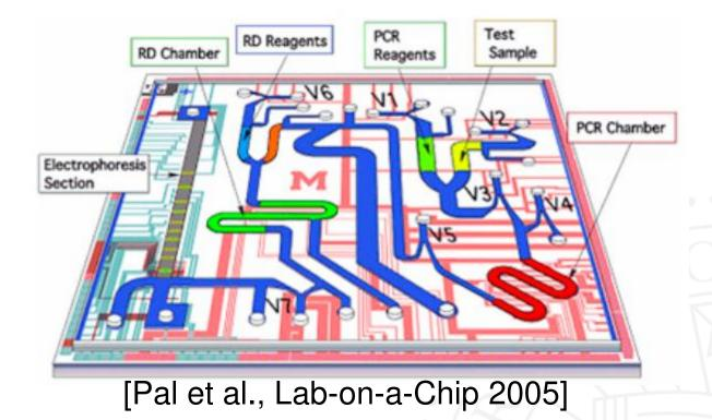
The thermocycling protocol applied to the device consists of 92 degrees C for 30s, and then 35 cycles of the following: 92 degrees C for 5s, 55 degrees C for 10s, and 72 degrees C for 20s, and finally 72 degrees C for 60s, for a total cycling time of 22 minutes. A portion of the PCR product (~60nl) is subsequently subjected to a restriction endonuclease digestion within the same device. The restriction digest reaction is performed at 37 degrees C for 10 min.
