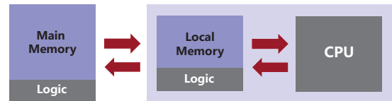
Figure 1. Logic-in-Memory Computing Paradigm: application-specific logic for localized computation is hidden behind a memory abstraction.
