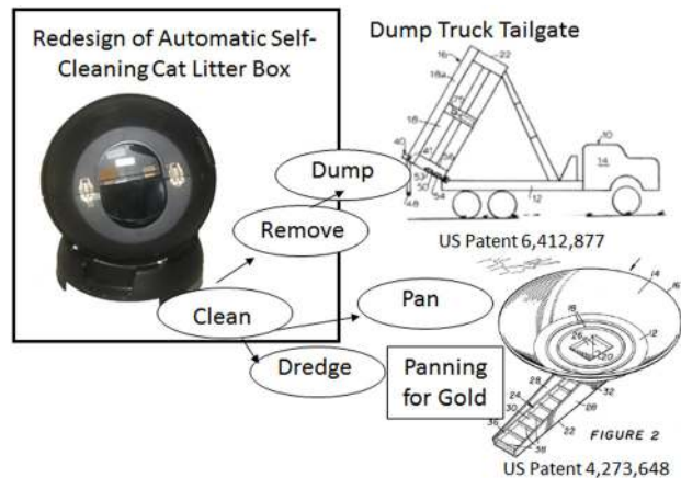
Fig. 15 Analogies and analogous domains identified by a team who was redesigning a self-cleaning cat litter box
