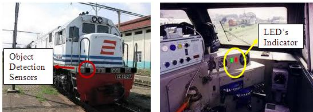
(A) (B) Figure 5. A. The object detection sensor is mounted on the front of the train head B. The LED indicators are placed on the driver room.
