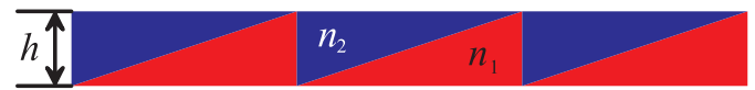
FIG. 3 Schematic representation of a DOE with common depth h , where the air between the sawtooths of a conventional blaze profile is substituted by a second material with another dispersion n_2(\lambda) .
