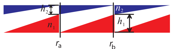
FIG. 4 Schematic representation of a multilayer DOE consisting of two sawtooth profiles of different materials together with paths in r_a and r_b at the boundaries of a local zone width d = |r_a - r_b| to determine optical path difference. r_a and r_b denote positions located near both sides of the discontinuities of the sawtooth profiles.
