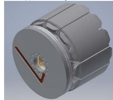
(b) Busbars assembled with machine Fig. 6. 3D representation of bus bars.
