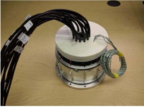
(b) Full assembly Fig. 7. Bus bars assembly.
