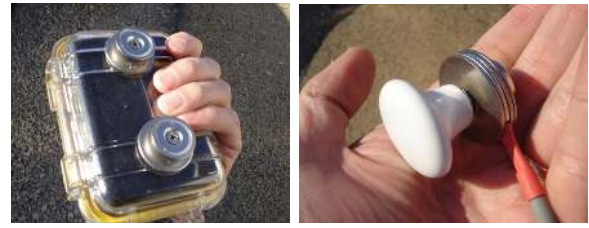
Fig. 3. RTDs attached to magnets at the base of the node enclosure (left) and an external magnetic RTD probe (right).
