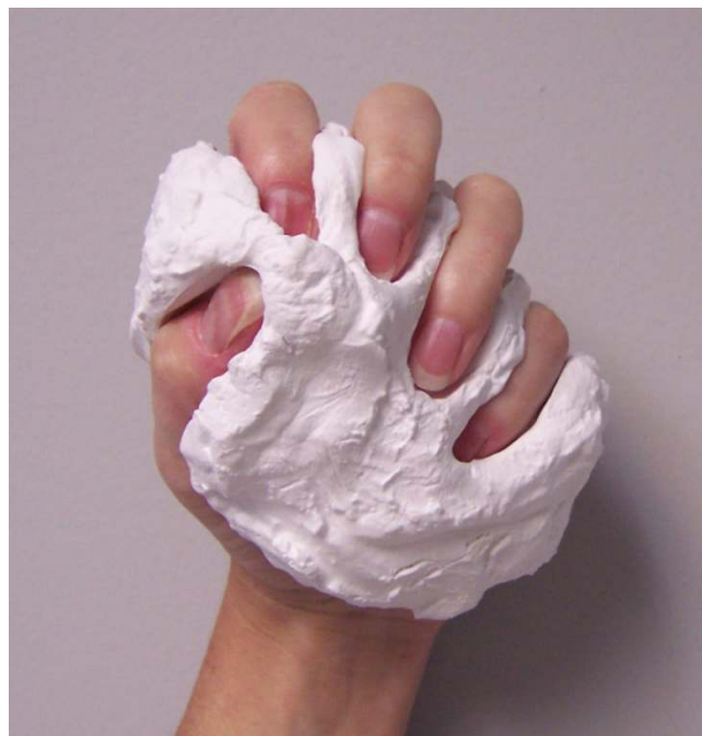
Figure 4 Grip mold. The grip mold is custom made for each subject. It provides a repeatable position for the fingers to assume for multiple grip-release activities in order to evaluate repeatability of measurement.
