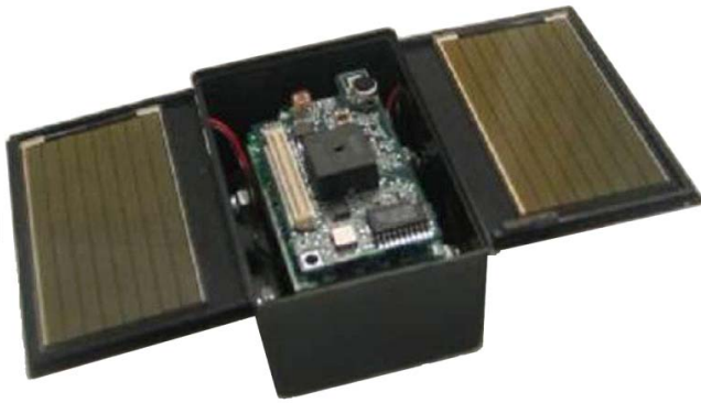
Fig. 3. Helimote, a solar harvesting sensor node.
