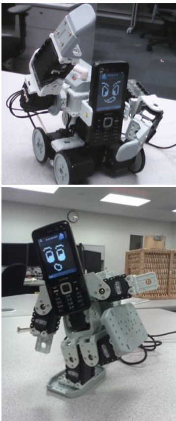
Figure 1. CALLY (top; the first generation prototype) and CALLO (bottom; the second prototype).
