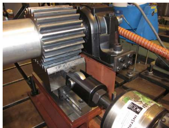
Figure 11. Rack and pinion gear power transmission system.
