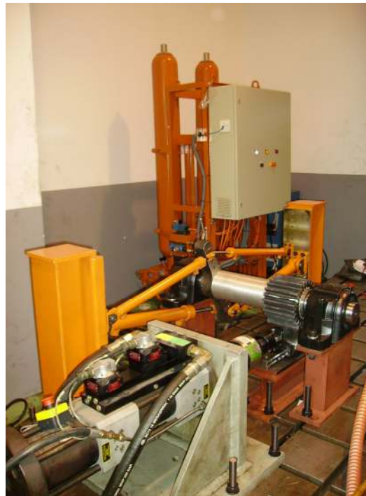
Figure 11. Rack and pinion gear power transmission system.
