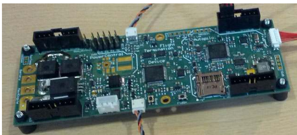
FIGURE 22 All central electrical functions of the DelftaCopter are integrated into a single board PCB for minimal weight and minimal interconnection failure. The four corner connectors lead to the systems in all four wings. From left to right, the board contains power, flight termination, and autopilot
