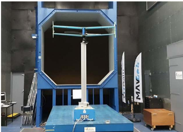
FIGURE 16 DelftaCopter in the Open Jet Wind tunnel of TUDelft. The tunnel outlet measures 2.85 \text{ m} \times 2.85 \text{ m} and can reach 30 \text{ m/s} wind speeds. DelftaCopter was mounted on a 1.8\text{-m} aluminum pole, which was standing on a force and moment balance. The Y-axis of the balance points into the tunnel opening. The X-axis points right in the picture and the Z-axis up
