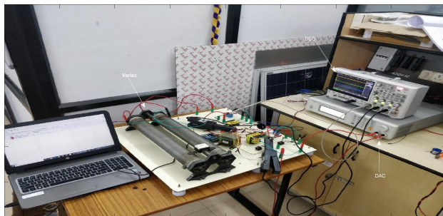
FIGURE 14: MPPT Experimental Setup for Color Spectrum
