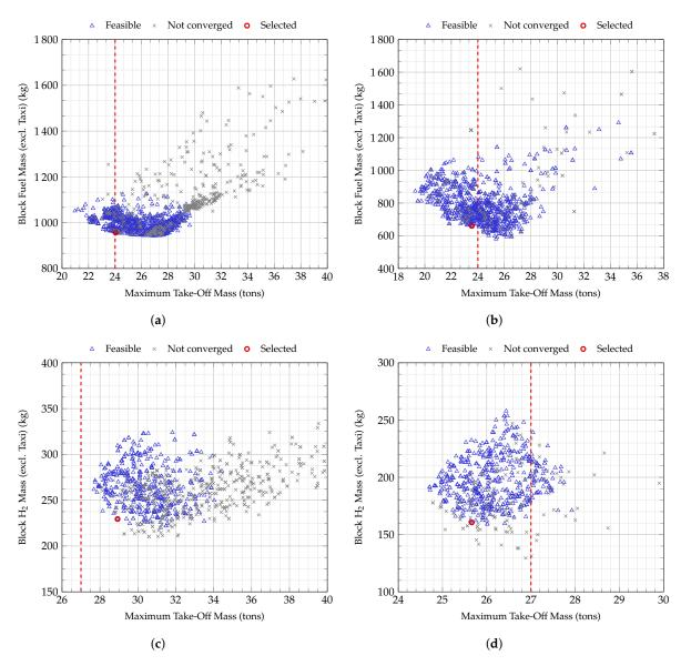
**Figure 8.** Selected values for DOE independent variables. Red dotted lines indicate the recommended upper threshold of the MTOM for the different scenarios. (a) Short-term ICE + battery. (b) Medium-term ICE + battery. (c) Medium-term PEMFC + battery. (d) Long-term SOFC + battery.
