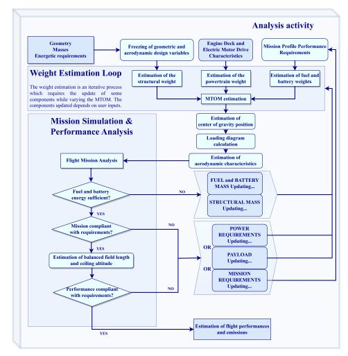
Figure 3. Workflow of the analysis module of HEAD.
