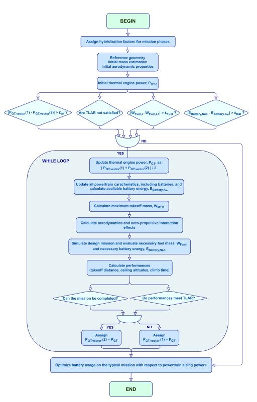
Figure 5. Detailed aircraft design workflow based on mission simulation.
