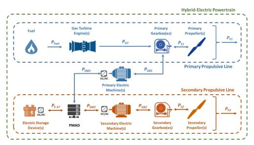
**Figure 1.** Example of a hybrid-electric propulsive scheme based on gas turbine engines and electric storage devices.
