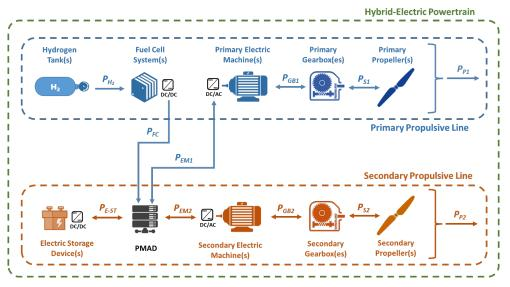
**Figure 2.** Example of a hybrid-electric propulsive scheme based on hydrogen-based fuel cells and electric storage devices.
