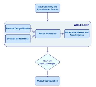
Figure 4. Simplified aircraft design workflow based on mission simulation.
