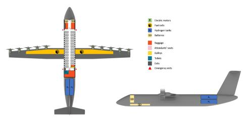
Figure 7. Schematic representation of the FC-based hybrid-electric configuration considered.
