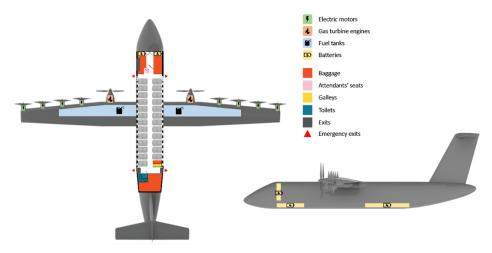
Figure 6. Schematic representation of the ICE-based hybrid-electric configuration considered.
