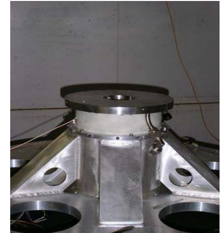
HTS Stability Bearing Cryostat Installed in DOE 5 kWh Flywheel
