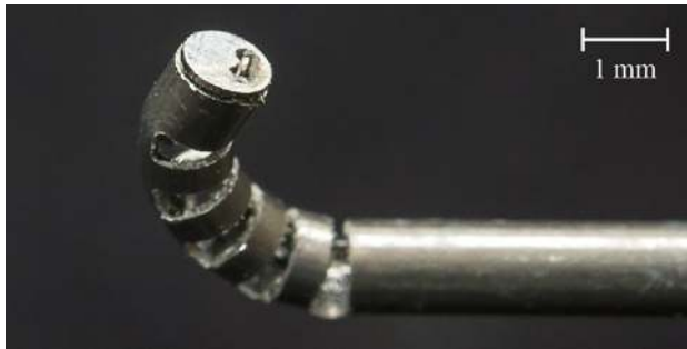
Fig. 9 The use of an end cap to attach the tendon to the tip of the wrist is shown. This is the tendon attachment method used in this work.
